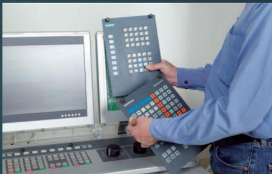
The conversion to another control system is carried out within a minute by calling up the respective software and by simply replacing the controller specific module.
